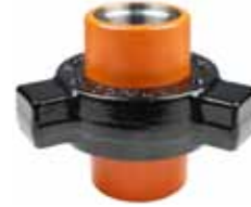
Figure 602 Threaded 6000 PSI CWP Specially Designed Lip Type Elastomer Seal Protects Metal to Metal Sealing Surface and Reduces Line Flow Turbulance
